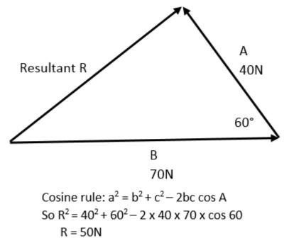
When the resultant vector has been found, it can be resolved into its horizontal and vertical components. For a vector of magnitude F, at an angle of *i* degrees above the x axis, the component in the x direction,  $F_x$ , is F cos *i*, and the component in the y direction,  $F_y$ , is F sin *i*.
